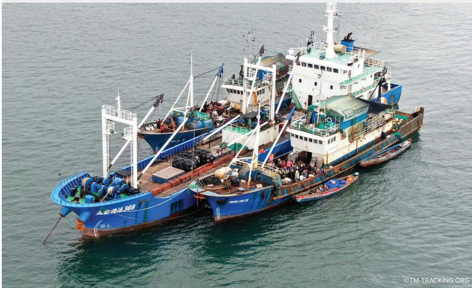
3. In some fisheries, "carriers" may come in the form of other fishing vessels, or even large canoes, but are normally large-sized steel-hulled refrigerated cargo (reefers), ships such as the middle vessel above between two trawlers
