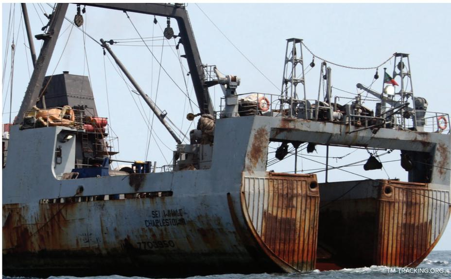
When not in use, otter boards will often be visible at the stern of a trawler (for those that use otter boards). If no doors can be seen, the vessel will probably be trawling, and the warps should be visible running from the towing or trawl blocks into the water astern of the vessel.
