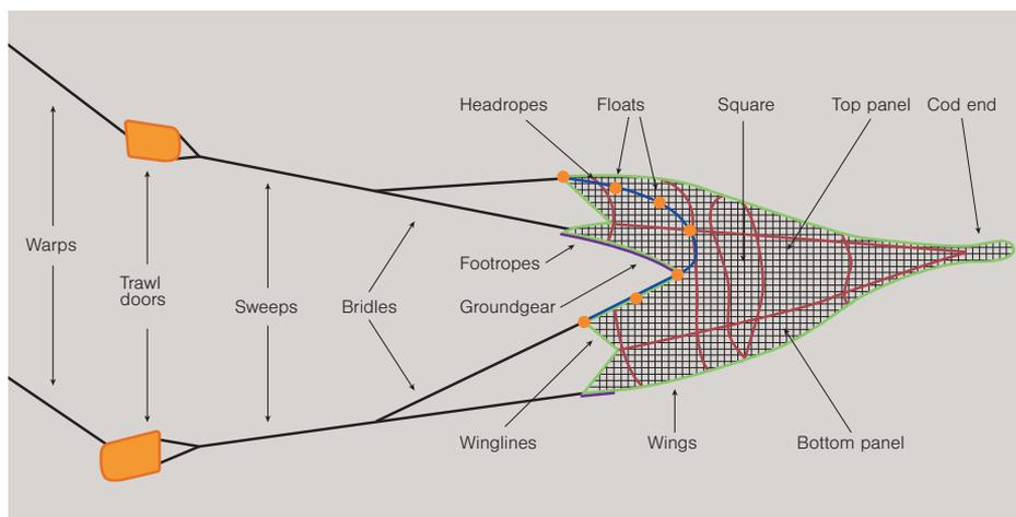
Figure 1. Overview of a trawl gear setup
