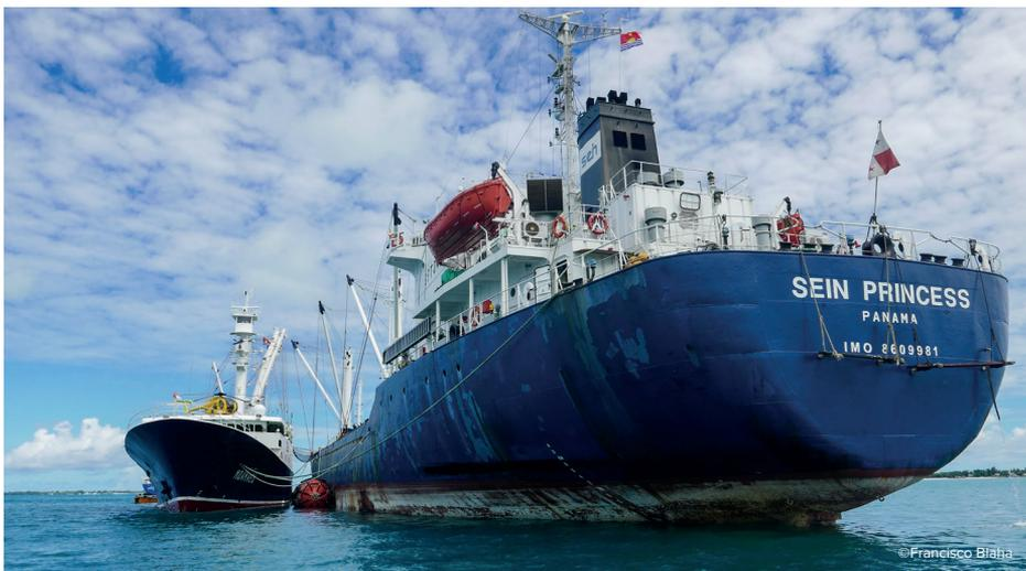
Transshipping at anchor in port area. Note the large 'Yokohama' fender deployed between the carrier and unloading vessel.
