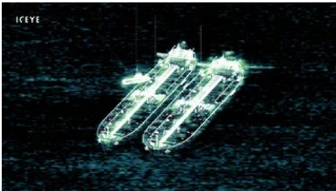
Figure 5. 'Dark rendezvous' transshipment by two tankers not emitting AIS signals, captured by SAR sensors and visualised in 3D. (Source: ICEYE)
