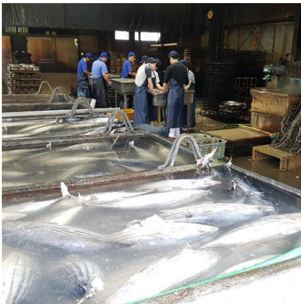
Thawing skipjack awaiting initial processing for katsuobushi in a small processing plant, Yaizu Photo: Tony Lewis
